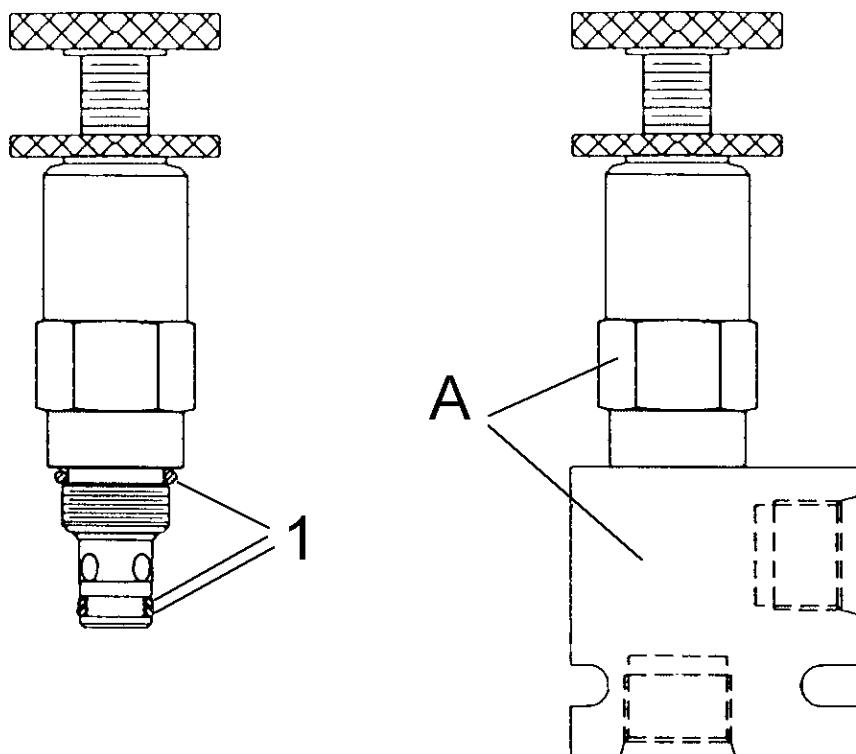
**WEIGHT TRANSFER VALVE****LIST OF PARTS****Hydra Force RV08-20**
